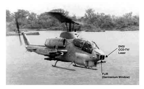
Figure 3-6. AH-1W with the NTS.
