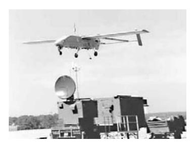
Figure D-2. Pioneer UAV Aircraft with GCS.
