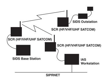
Figure 3-8. Manpack SIDS Communications Connectivity.
