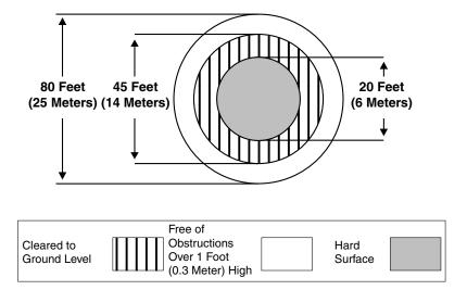
Figure G-5. Small Landing Point Dimensions.
