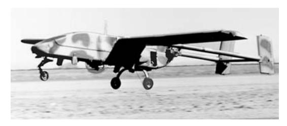
Figure D-1. Pioneer UAV Aircraft.
