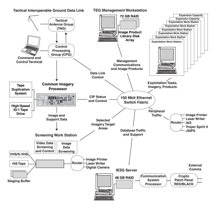
Figure 4-18. IIP/TEG Systems Architecture.
