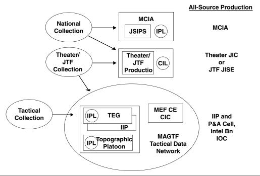
MCIA (which operates the JSIPS) and the IIPs (which will operate the TEG in each MEF architecture) are the Marine Corps' principal imagery and IMINT processing and production facilities. Within the MEF, the principal all-source intelligence processing and production agency is the Production and Analysis Cell, Intelligence Battalion.
